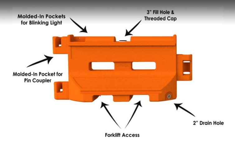
The GUARDSAFE® 36 barricade is a water-filled Longitudinal Channelizing Device (LCD) ideal for traffic and pedestrian channelization in almost any environment. The barricade is manufactured with rotationally-molded polyethylene, which allows it to withstand the harshest weather conditions and resist dents and cracks.
